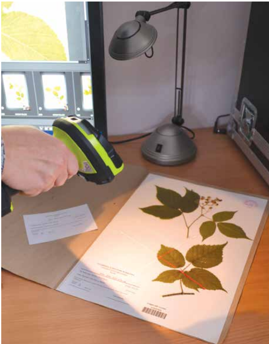
Fig. 3. The barcode reader helps an operator in managing the data
